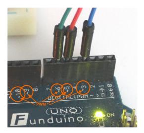
The PWM lets the voltage pulse from +5V to 0V. So the voltage gets turned off and on for only milliseconds. With a really high PWM the 5 V signal nearly gets constant on the pin. With a low PWM it is the other way around and the 5 V signal is barely there (This is only a reduced summary, so you should look it up on the internet, if you need more information). With PWM it is possible to get nearly the same effect as if the voltage would vary.
