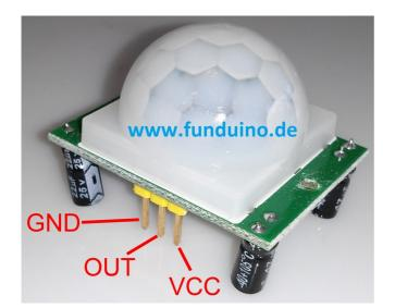
The plastic lens on top of the motion detector can easily be removed. Underneath of it, there is the IRdetector and the lettering of the three contacts. GND ( - ), OUT (Signal output), VCC ( + ).
