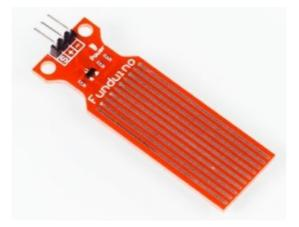
One example of the usage can be a rain detector. If the drop sensor measures a rain drop, the Arduino board could e.g. close the blinds, set off an alarm or turn on windshield wipers.
