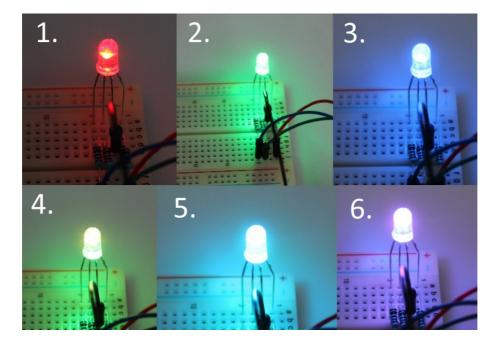
There is a simple way to find out what RGB LED version you have. Just switch "+" and "-" on the LED. Only if the LED is connected the right way it will work and shine.
