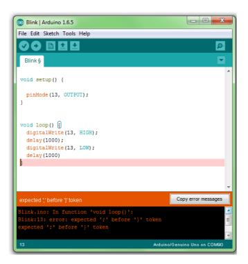
2.) There is a mistake in the sketch. For example, a word is misspelled or a bracket is missing. In the example on the left the last semicolon in the sketch is missing. In this Case the error report often starts with "excepted..". This means that the program is still expecting something that is missing.
