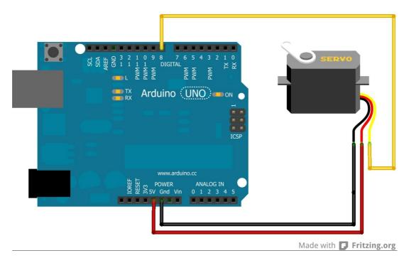
Required equipment: Arduino / one servo / three cables
