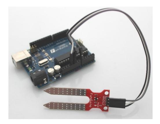
The programming of the moisture sensor isn't that complicated and is very similar to the programming of the potentiometer, because there is just an analog value read out.
