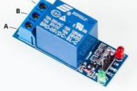
The relay needs a permanent power supply trough 5V+ and – (In the picture VCC and GND). With the "IN"-pin, the switch can be activated by the Arduino board. The three terminals on the left side are meant to be connected with the electrical component that needs more power than the Arduino can provide. If the relay doesn't get any signal from the Arduino on the "IN" contact, the contacts A and B are connected. Once the relay gets a signal from the Arduino the contacts B and C get connected.
